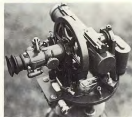
The theodolite operator is a key member of the flight inspection team. The theodolite provides a visual cross-check of aircraft position. This helps ensure the in-flight check is accurate.
