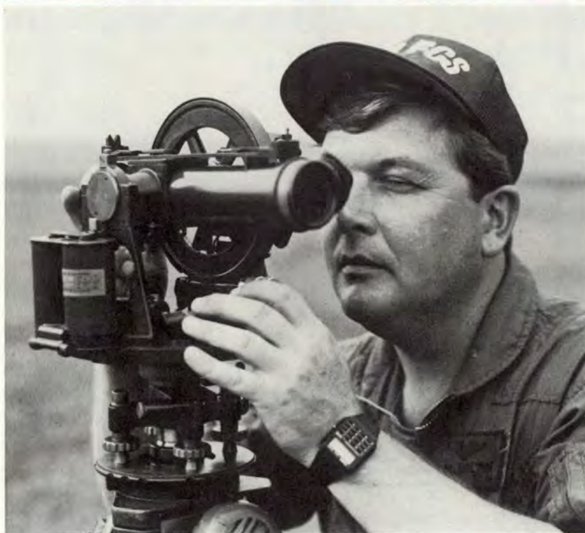
The theodolite operator is a key member of the flight inspection team. The theodolite provides a visual cross-check of aircraft position. This helps ensure the in-flight check is accurate.
