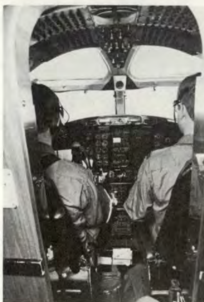
Accurate flight checks of NAVAIDS and precision landing systems are dependent on the entire crew. The pilots must fly the aircraft precisely while the technician uses special equipment to monitor, record, and analyze the transmitted signal.
